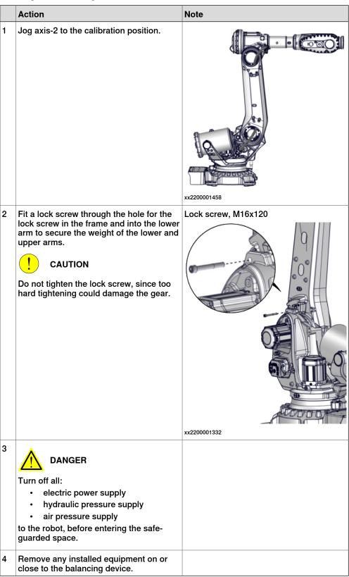
Unloading the balancing device springs and locking position with the Hydraulic press equipment, balancing device
