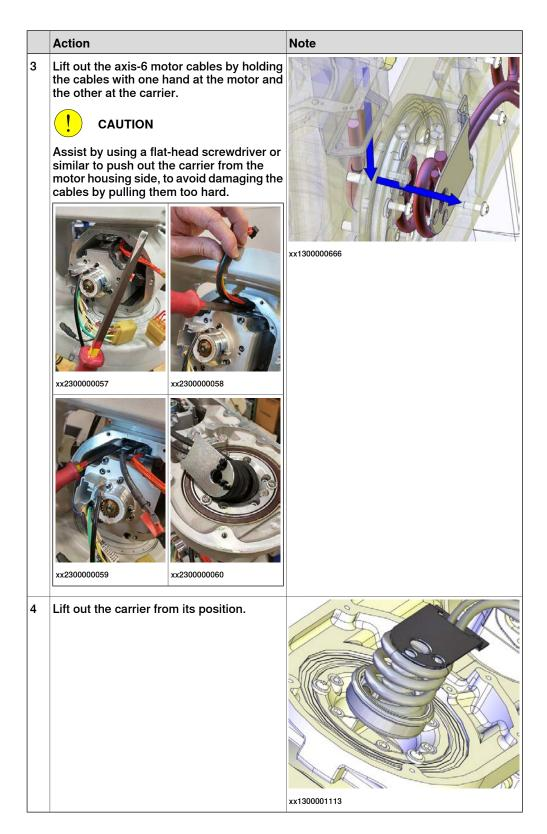
5.4.1 Replacing the arm house cover including the axis-4 cassette sealing *Continued*
