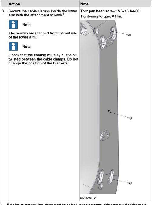
If the lower arm only has attachment holes for two cable clamps, either remove the third cable bracket from the spare part cable harness, or drill attachment holes in the lower arm. Contact ABB for more information.
