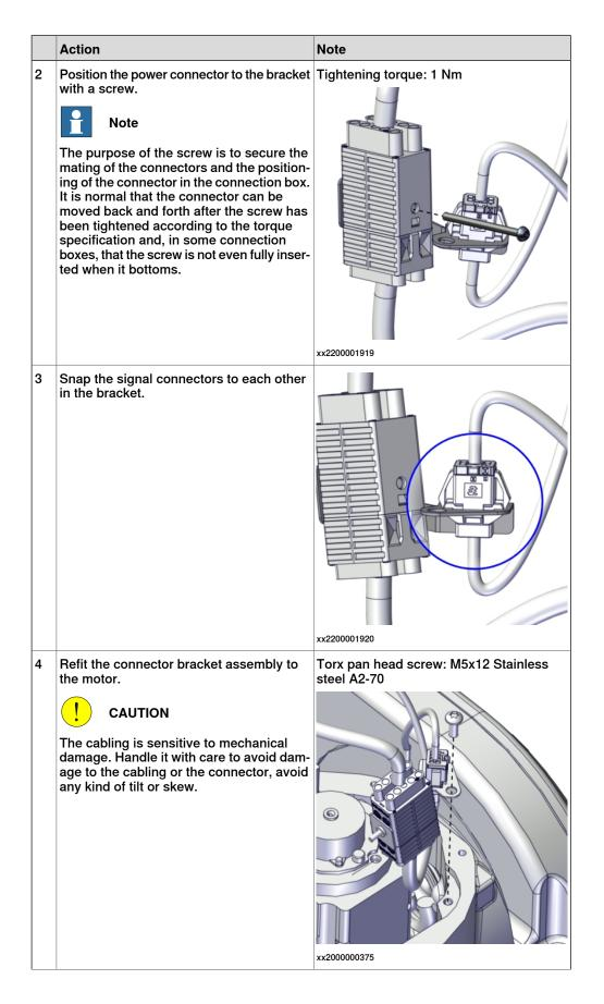
5.8.3 Replacing the axis-3 gearbox *Continued*
