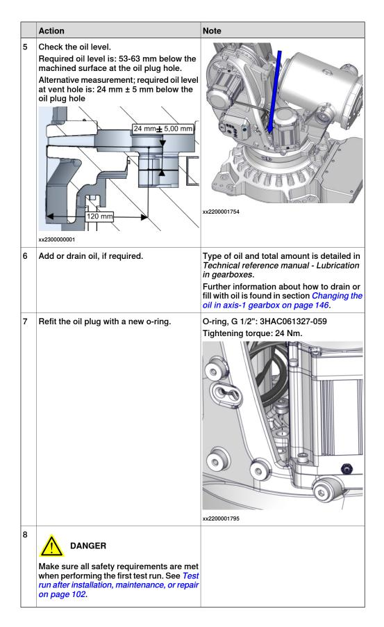
4.3.8 Inspecting the oil level in axis-2 gearbox
