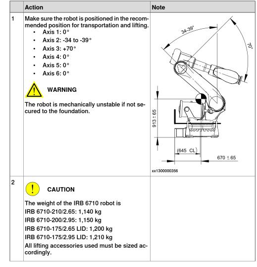
3.3.3.3 Lifting the robot with roundslings *Continued*
