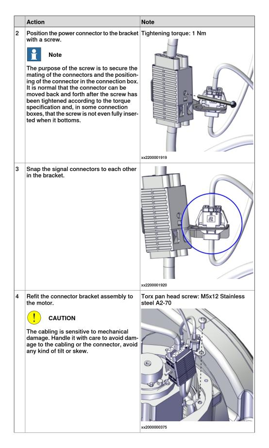
5.8.4 Replacing the axis-6 gearbox *Continued*
