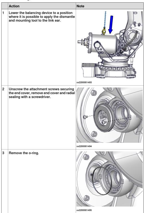
5.3.2 Replacing spherical roller bearing, balancing device link ear *Continued*
